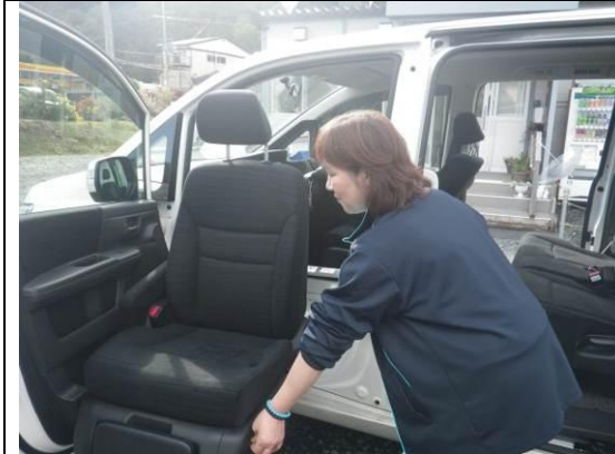
The manager of a home for elderly in Yasuragi demonstrates how to use a movable front passenger seat. This function makes it possible for the staff to lift the clients without strain into a car and relieves their hesitation about going out. © JRCS
