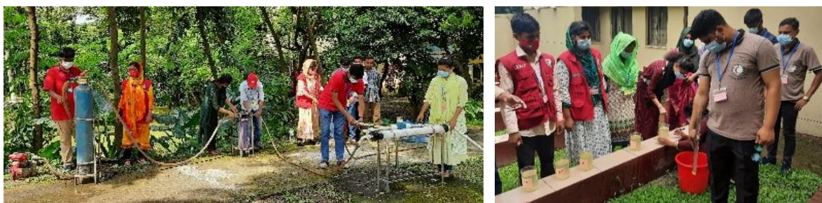
Participants setting up and running the Man-pack (left) and carrying out jar test to determine optimal coagulant dose (right) (Photos: BDRCS)
