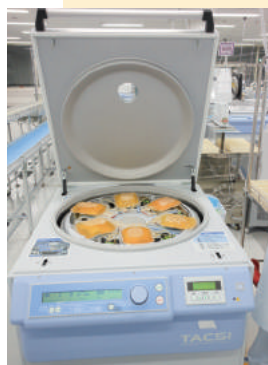
Automatic Centrifuge and Separator Integration (Whole Blood to Blood Components)
