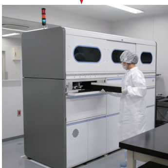
NAT screening (extraction of nucleic acids, amplification and detection of viral nucleic acids)
